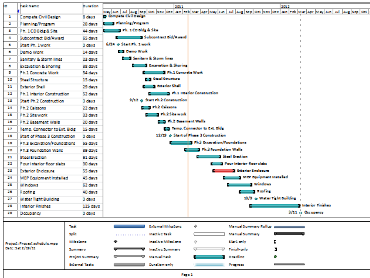
Accelerated Critical Path Schedule, No overall change (Red shows the change for SlenderWalls)
